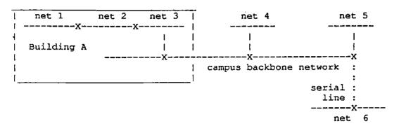
Nets 1, 2 and 3 are in one building. Nets 4 and 5 are in different buildings on the same campus. Net 6 is in a somewhat more distant location. The diagram above shows nets 1, 2, and 3 being connected directly, with switches that handle the connections being labelled as "X". Building A is connected to the other buildings on the same campus by a backbone network. Note that traffic from net 1 to net 5 takes the following path:
