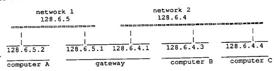
Note that the gateway has IP addresses assigned to each interface. The computers' routing tables are set up to forward through appropriate address. For example, computer A has a routing entry saying that it should use the gateway 128.6.5.1 to get to subnet 128.6.4.
