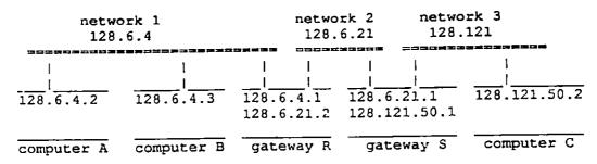
This diagram shows three normal computer systems, two gateways, and three networks. The networks might be Ethernets, token rings, or any other sort. Network 2 could even be a single point to point line connecting gateways R and S.
